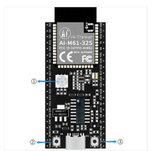
Figure 5 Ai-M61-32S-Kit indicator light and key position
