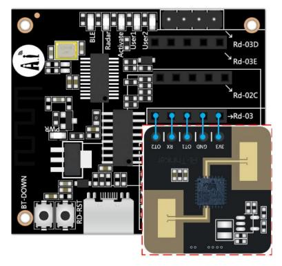
Figure8 Schematic diagram of Rd-03/03L wiring
