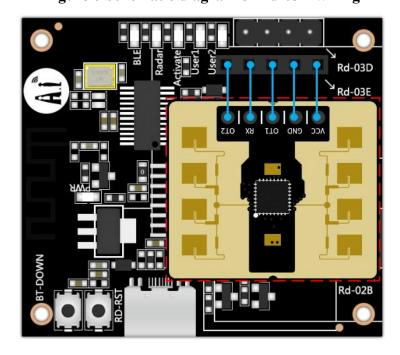
Figure 7 Schematic diagram of Rd-03E wiring
