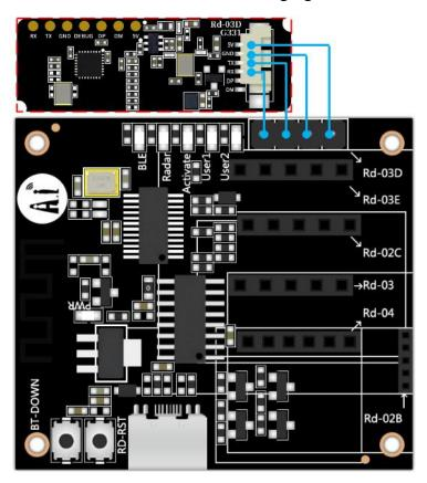
Figure 6 Schematic diagram of Rd-03D wiring
