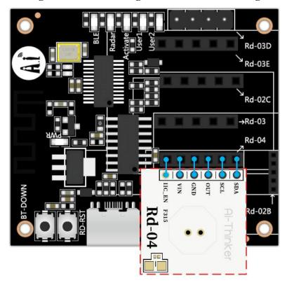
Figure 9 Schematic diagram of Rd-04 wiring
