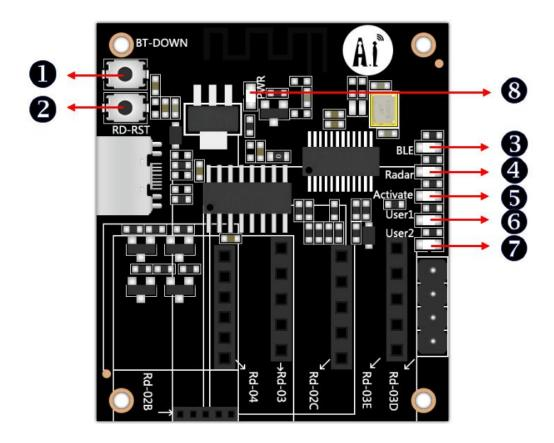
Figure 5 Rd-Kit indicator light and key position
