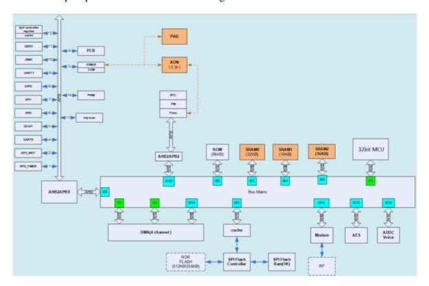
Figure 1 Main chip block diagram
