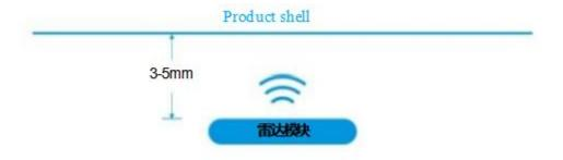
Figure 9 Distance between antenna surface and product shell
