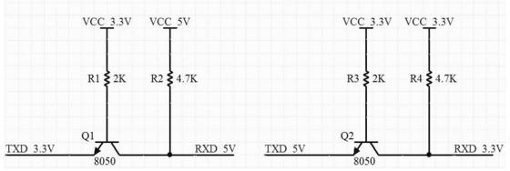
Figure 14 level conversion circuit
