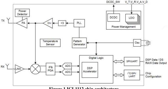
Figure 1 ICL1112 chip architecture
