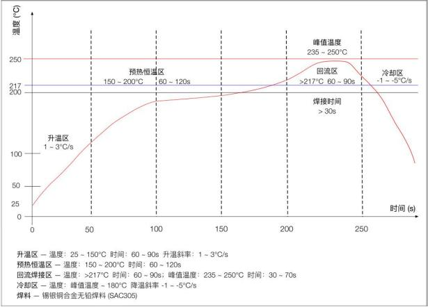
Figure 15 Reflow welding curve
