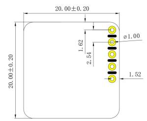
Figure 9 recommend PCB package size
