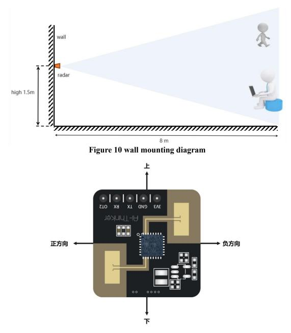
Figure 11 schematic diagram of wall hanging direction
