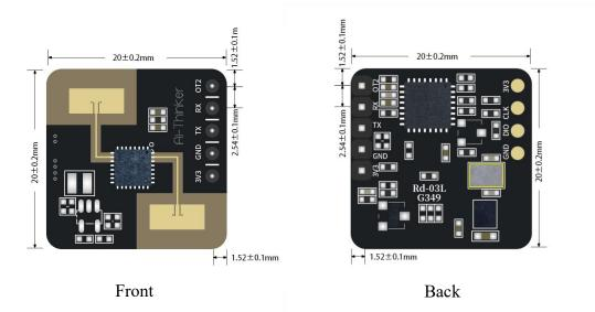
**Figure 5 Dimension Diagram**
