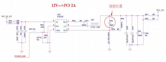
Figure 13 DC-DC step-down circuit diagram
