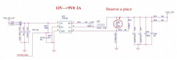
Figure 14 DC-DC step-down circuit diagram
