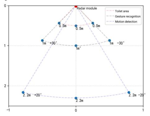
Figure 13 Gesture recognition hanging wall radar power diagram
