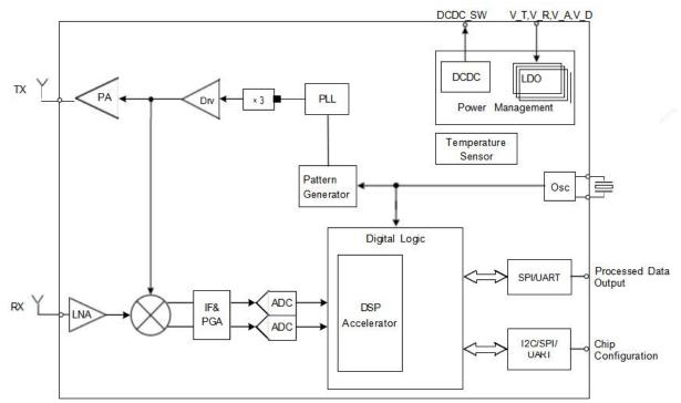
Figure 1 S3KM111Larchitecture diagram
