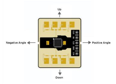
Figure 12 Schematic diagram of gesture recognition detection range
