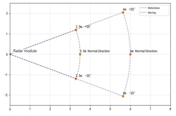
Figure 10 Power map of precision ranging wall-mounted radar
