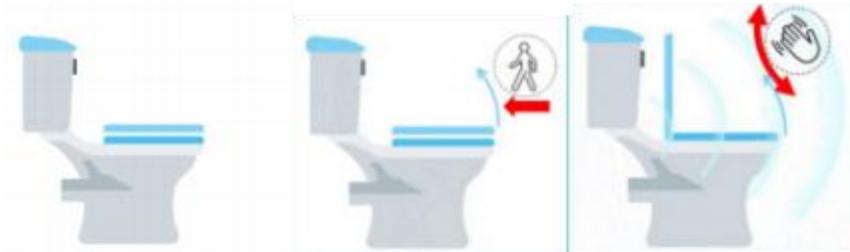
(a) No one state (b) People come to open the cover (c) Gesture circle turning
