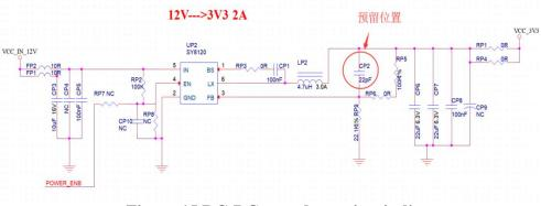
Figure 15 DC-DC step-down circuit diagram
