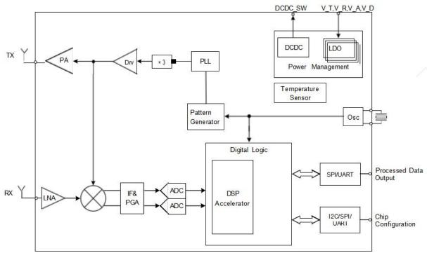
Figure 1 S3KM1110 architecture diagram
