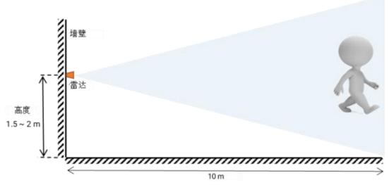
Figure 12 Schematic diagram of wall mounting
