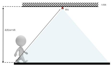
Figure 9 Schematic diagram of mounting the roof
