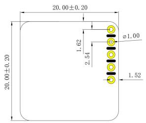
Figure 8 Recommended PCB package size
