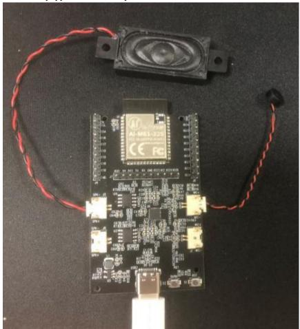
The function of the firmware is to play the microphone input sound in real time through the speaker.
