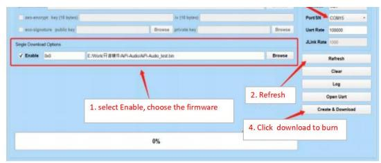
**Note:** After the firmware is burned, you need to press the reset button for one time, then the program can be run.
