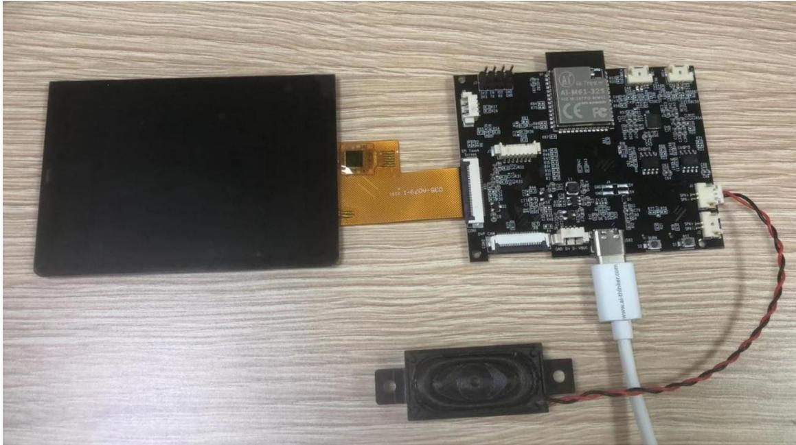
Connect the screen, speaker, Type-C cable to the board
