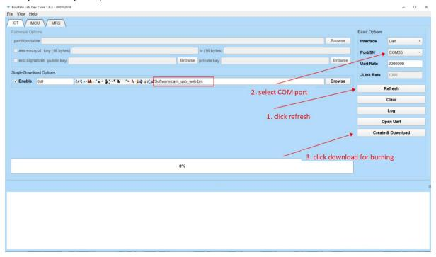
**Note:** After the firmware is burned, you need to press the reset button for one time, then the program can be run.
