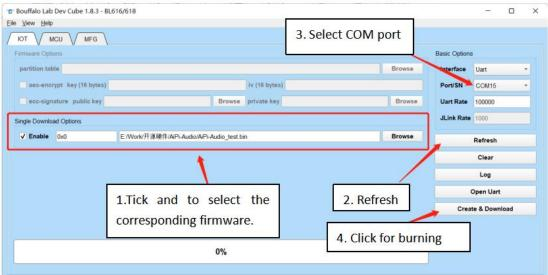
Note: After the firmware is burned, you need to press the reset button once before the program can run.
