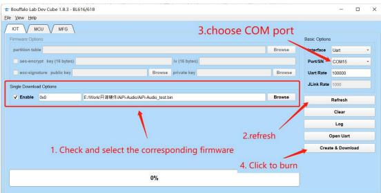
Note: After the firmware burning is completed, you need to press the reset button once before the program can run.
