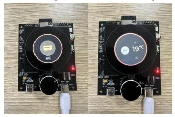
Standby: When the power is turned on, if no operation is performed for a period of time, the standby mode will be automatically entered. At this time, a dynamic screen protection wallpaper will appear. If you press the knob arbitrarily, the standby mode will be exited and the state before standby will be entered.
