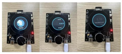
The second is the TV control end, short press to enter the TV station selection interface, rotate the knob and short press to select the station, at this time the remote control interface is displayed, there are various buttons, you can rotate and short press the knob to select, key buttons include volume adjustment, channel adjustment, etc. Hold down to exit the current screen.
