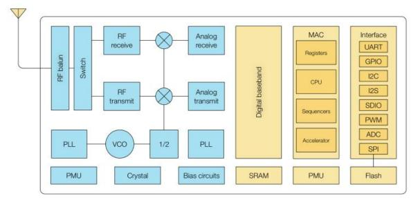
ESP8266 has a complete and self-contained Wi-Fi network function, which can be used independently or run as a slave on other host MCUs. When ESP8266 is applied independently, it can be started directly from external flash. The built-in cache memory helps improve system performance and optimizes the storage system.
