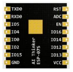
Figure 2.1 ESP-07S Pin diagram
