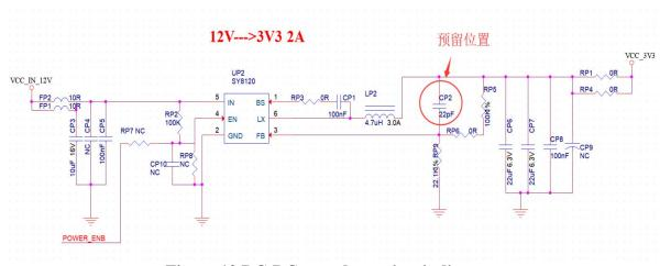
Figure 10 DC-DC step-down circuit diagram
