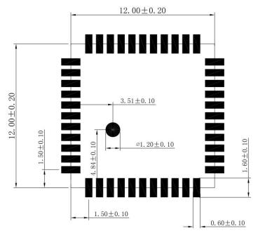
Figure 9 Recommended PCB package sizes (unit: mm)
