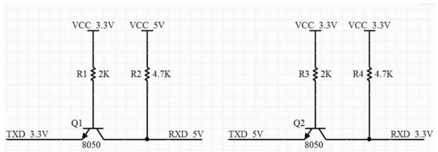
Figure 11 Electrical Level conversion circuit
