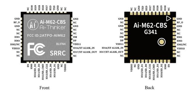
Figure 6 Schematic diagram of the module pin
