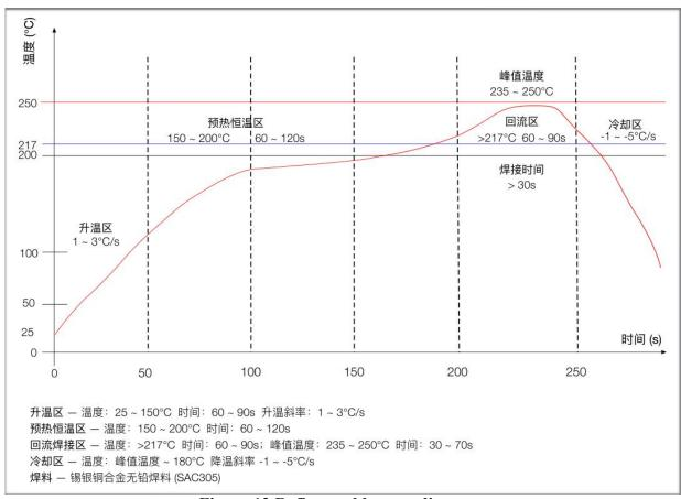
Figure 12 Reflow weld curve diagram
