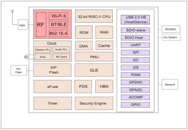
Figure 1 Main chip block diagram
