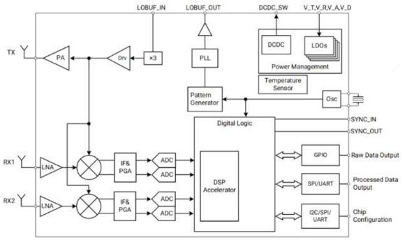
Figure 1 S5KM312CL architecture diagram
