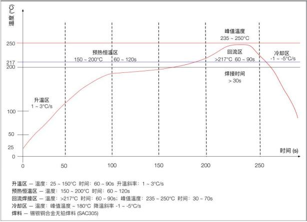
Figure 13 Reflow welding diagram
