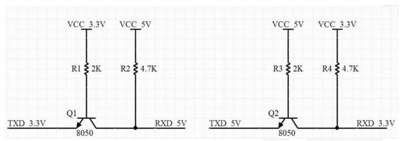
Figure 12 Level switching circuit
