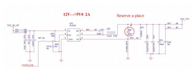
Figure 11 DC-DC buck circuit diagram
