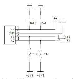
Figure 7 Application guide circuit
