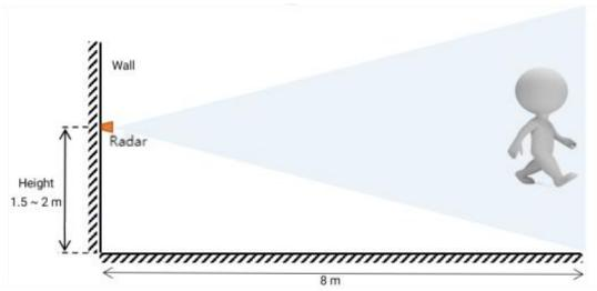
Figure 8 Wall mounting diagram
